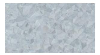
Galvalume is a long-lasting zinc-aluminum alloy spangle that offers superior corrosion resistance. Painted metal roof panels typically begin with Galvalume and are then primed and painted, but Galvalume alone looks amazing – from many angles it will look nearly white, in other angles more of a gray finish. Not as "shiny" as galvanized.
