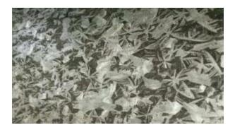
Galvanized roofs are the original – a 100% zinc coating with spangles that vary in size and shape.
